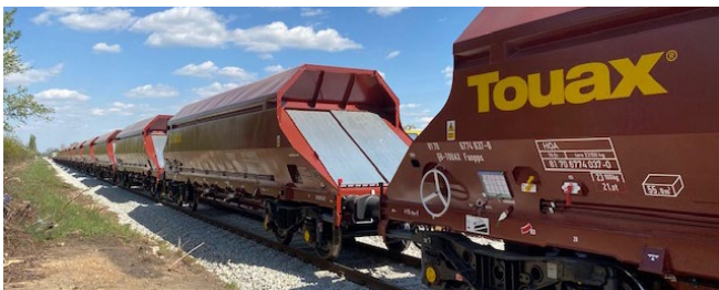
New built aggregate hoppers wagons for UK market
